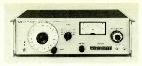
single-ended outputs of 50 and 750 impedance respectively. Maximum output is +11dB (2.5V into 6002), the precision attenuator has an 89-dB range in 1-dB steps, with an accuracy of 0.15dB on the higher ranges. The centre-zero output meter has an expanded scale with a range of -1 to +1dB, giving a 0.02-dB resolution for precise incremental adjustment of the output level. Price: £403. Hewlett-Packard Ltd, 224 Bath Road, Slough, Bucks. WW325 for further details
