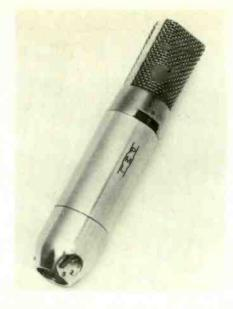
signal cable powering system, which permits the use of a screened twin cable to carry the microphone current (0.5 to 0.7 mA) and the output signal current. Suitable for all broadcasting and recording use, the unit measures  $150 \times 31$  mm, has stand adaption or can be hand-held. Jagor Interelectric Ltd, Mercury House, Hanger Green, Ealing, London W.5.
