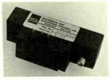
4.25GHz, tuning voltage of ± 15V or 0 to ± 30V, power output of 40mW minimum, input of 2W and operating temperature of -40 to +80°C. Phase-lock and crystal-controlled variants are also available. MESL, Lochend Industrial Estate, Newbridge, Midlothian, Scotland.
