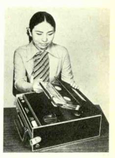
The Panasonic (Matsushita) magazine loading v.t.r. The unit is built to the specifications laid down in the Japanese Type I Standard for  $\frac{1}{2}$ -inch video tape recorders. The magazine illustrated contains enough tape for recording and reproducing a 30-minute programme.
